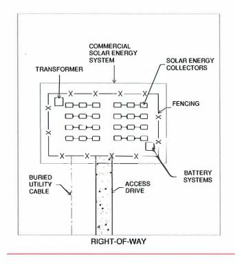
GROUND MOUNTED SOLAR ENERGY COLLECTOR: A solar energy collector that is not attached to and is separate from any building on the parcel of land on which the solar energy collector is located (Figure 1).
